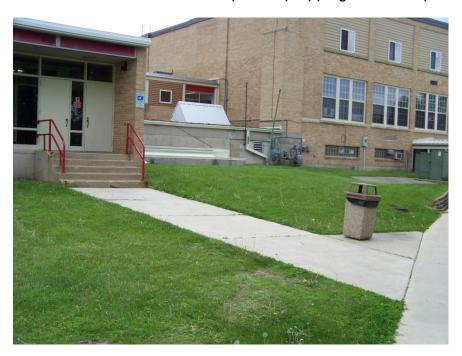
Install fence with a gate from the west wall face building wall by the steps over to the west side of the gas meter. Kill all the grass in the fenced area and install crushed rock for ease of maintenance. The fence will serve two functions: 1) The fence will limit anyone from being able to access the roof of the entire building from the low roof point 2) The fence will limit anyone from accessing the building utilities.
